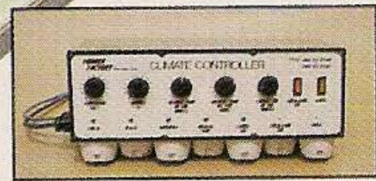
The Climate Controller commands watering, nutrients, air temperature, air movement, humidity and carbon dioxide levels and requires no user adjustment.
